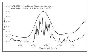
Figure 2: Comparison of NIST SRM 1920a spectra generated on an FT-NIR and dispersive instrument
