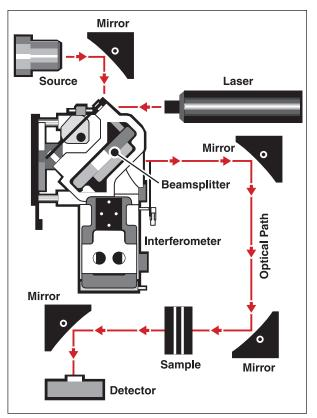
Figure 1: Illustration of spectrometer layout
