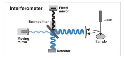
In addition to freedom from fluorescence interference, another advantage of FT-Raman spectroscopy is its exceptionally good x-axis (shifted wavenumber) accuracy as a result of the internal interferometer calibration supplied by the built-in helium-neon laser. Both of these attributes make FT-Raman the ideal technique for collecting spectra for reference libraries.
