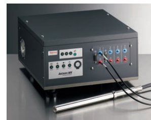
Antaris MX analyzer with process-rated reflection probe
