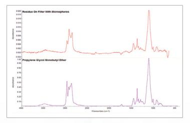
Figure 6: Even after several washes of the filter with water, some residual cream remains from the lotion as well as the particles.
