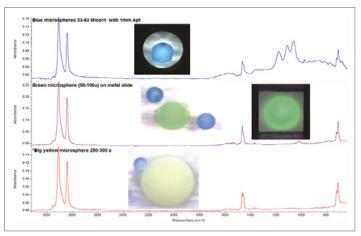
**Figure 7:** All three spheres are polyethyleene. However the spectrum from the small blue spheres contains a second component with strong peaks above 1000 cm<sup>-1</sup>. A spectral search of this region produces a good match for Barium Sulfate.
