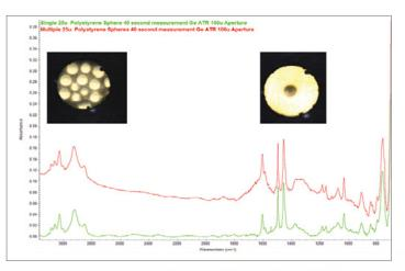
Figure 4: Beads through 100 micron aperture demonstrate 4X magnification with Germanium.
