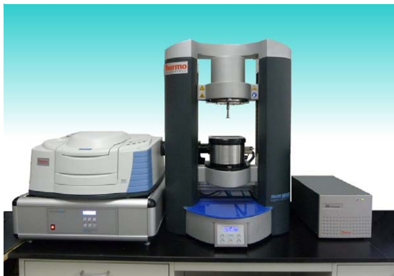
Fig. 1: The Thermo Scientific HAAKE MARS rheometer (centre) with a mounted Rheonaut module* connected to a Thermo Scientific Nicolet iS10 spectrometer (left).
