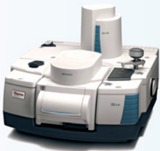
Thermo Scientific Nicolet iS50 FT-IR spectrometer with ABX Automated Beamsplitter exchanger, built-in diamond ATR, and Raman module in the sample compartment.
