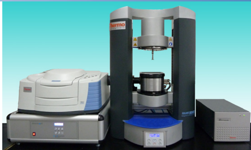
Modular rheometer platform Thermo Scientific HAAKE MARS III with Rheonaut module and Thermo Scientific Nicolet™ iS™10 FT-IR spectrometer
